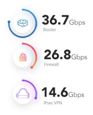
iperf3-bidir (32 Streams) tests were used to measure throughput. See our hardware comparison chart below for greater detail.
